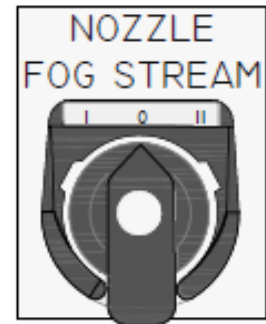
3-Position spring return to center selector switch.
