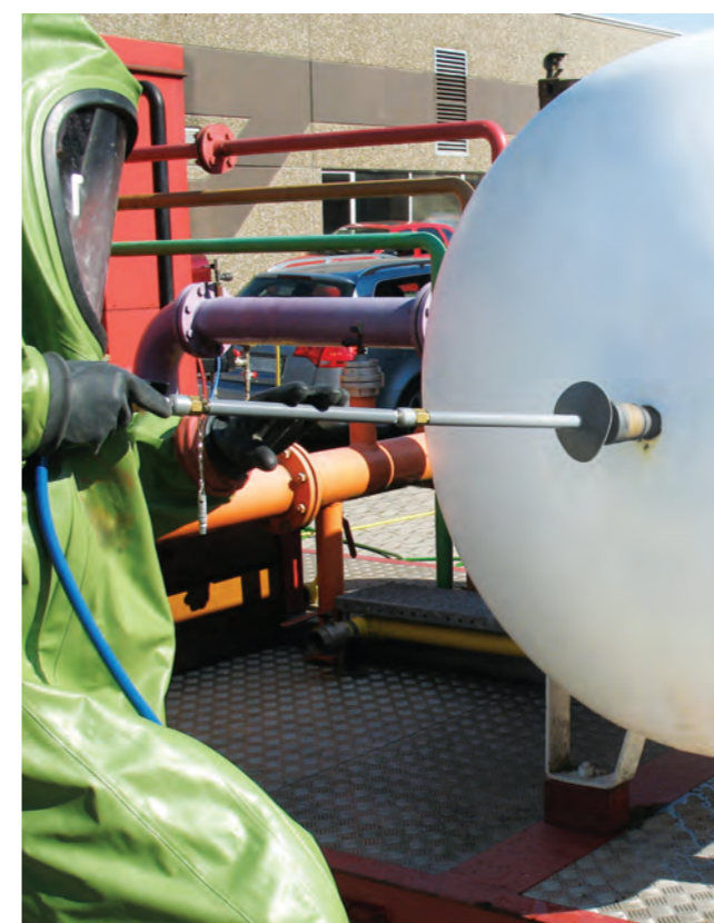
Seal leaks from a safe distance
