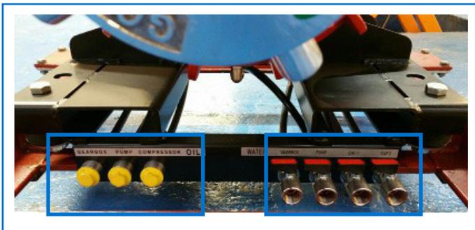
Gearbox/heat exchanger coolant and the CAFS manifold
