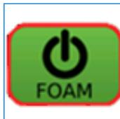
Foam concentrate is only injected when the foam button has the **RED** selector around the control button
