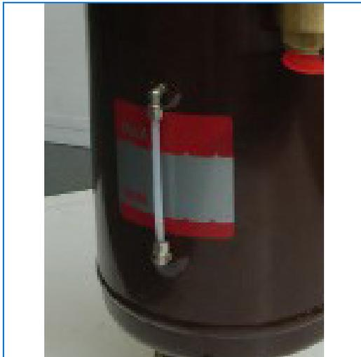
Separator tank - oil level indicator
