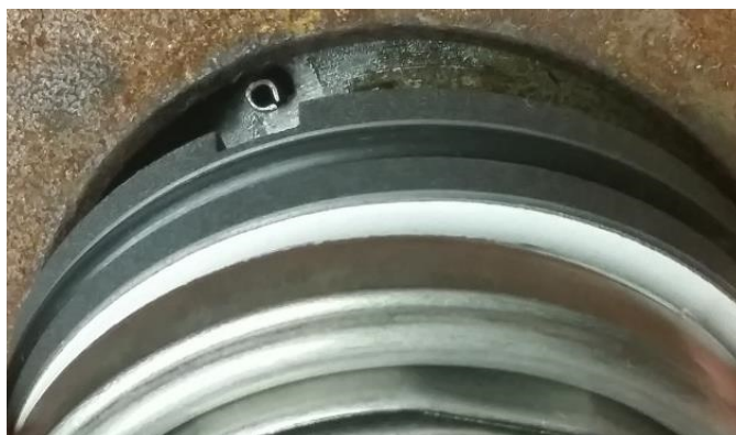
Figure 36. Align Slot On Seal With Pin In Pump Head
