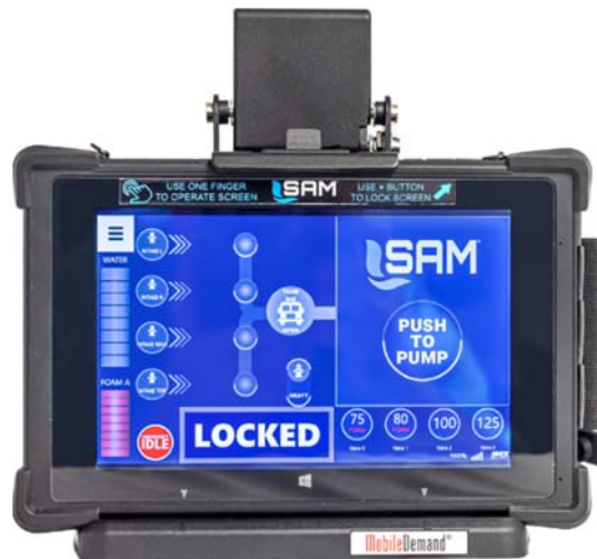
Figure 2. Emergency IDLE Activation (From A Locked Screen)
