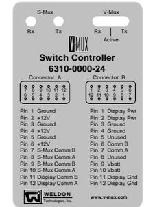
SWITCH CONTROLLER LABEL SHOWING CONNECTOR PIN ASSIGNMENTS
