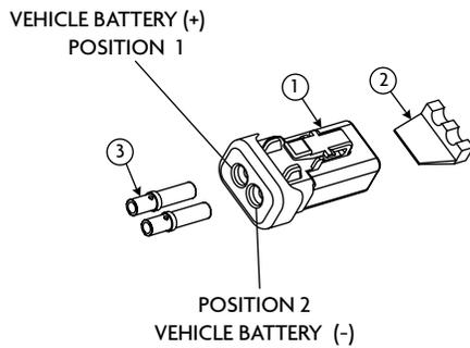
**Figure Z – CAN Connector**
