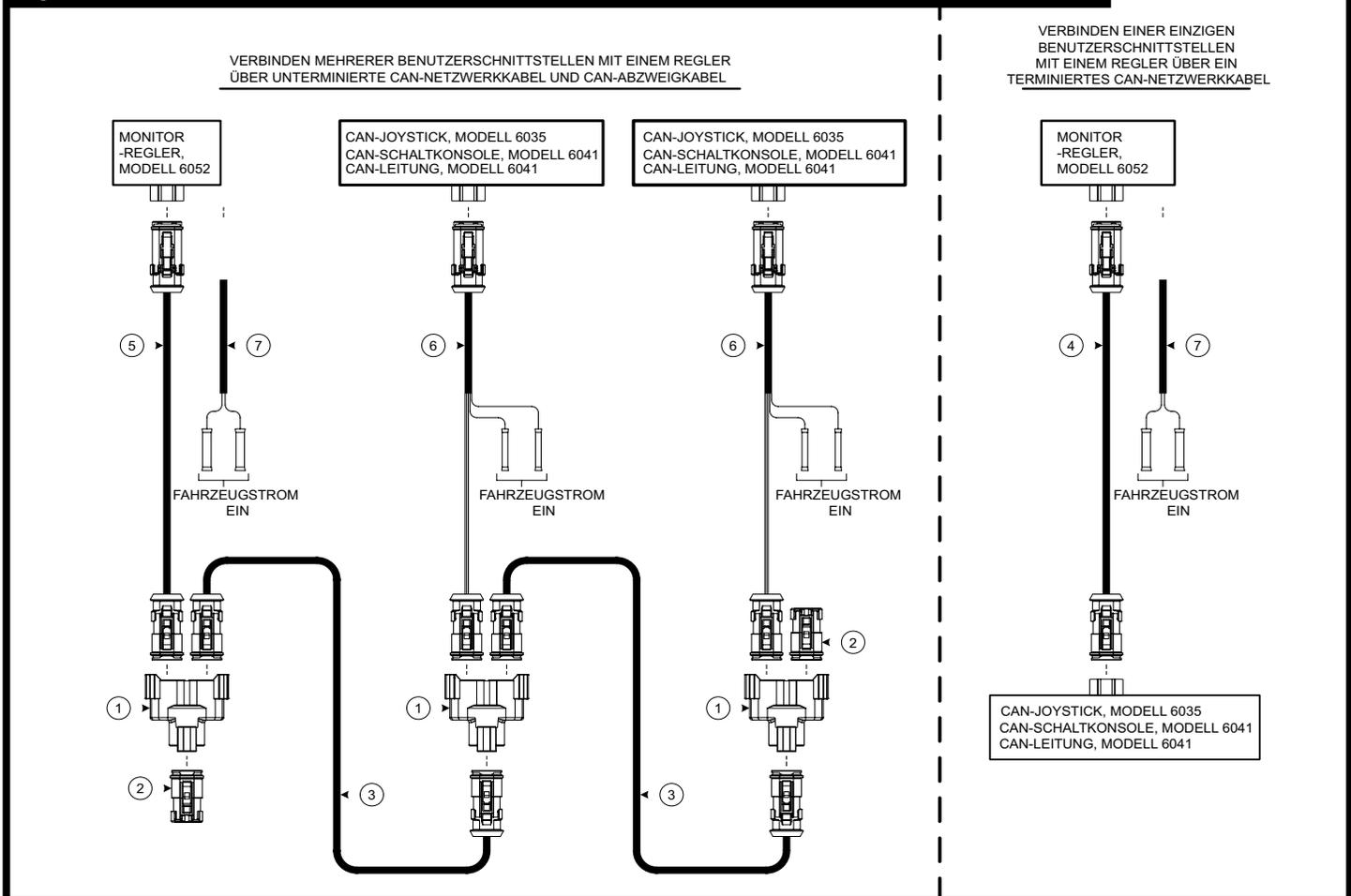
**MATING CONNECTORS FOR MONITOR CONTROLLER (See Figures Y and Z)**
