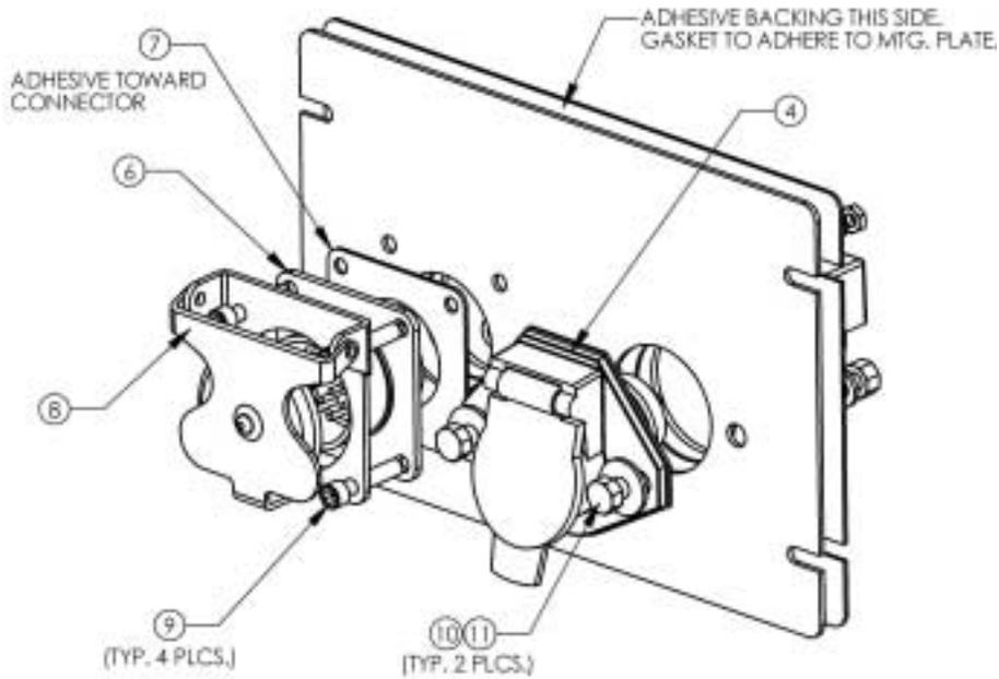
Figure 5 – 0N10-1037-00 Module Face Plate Sub-Assembly, Back side
