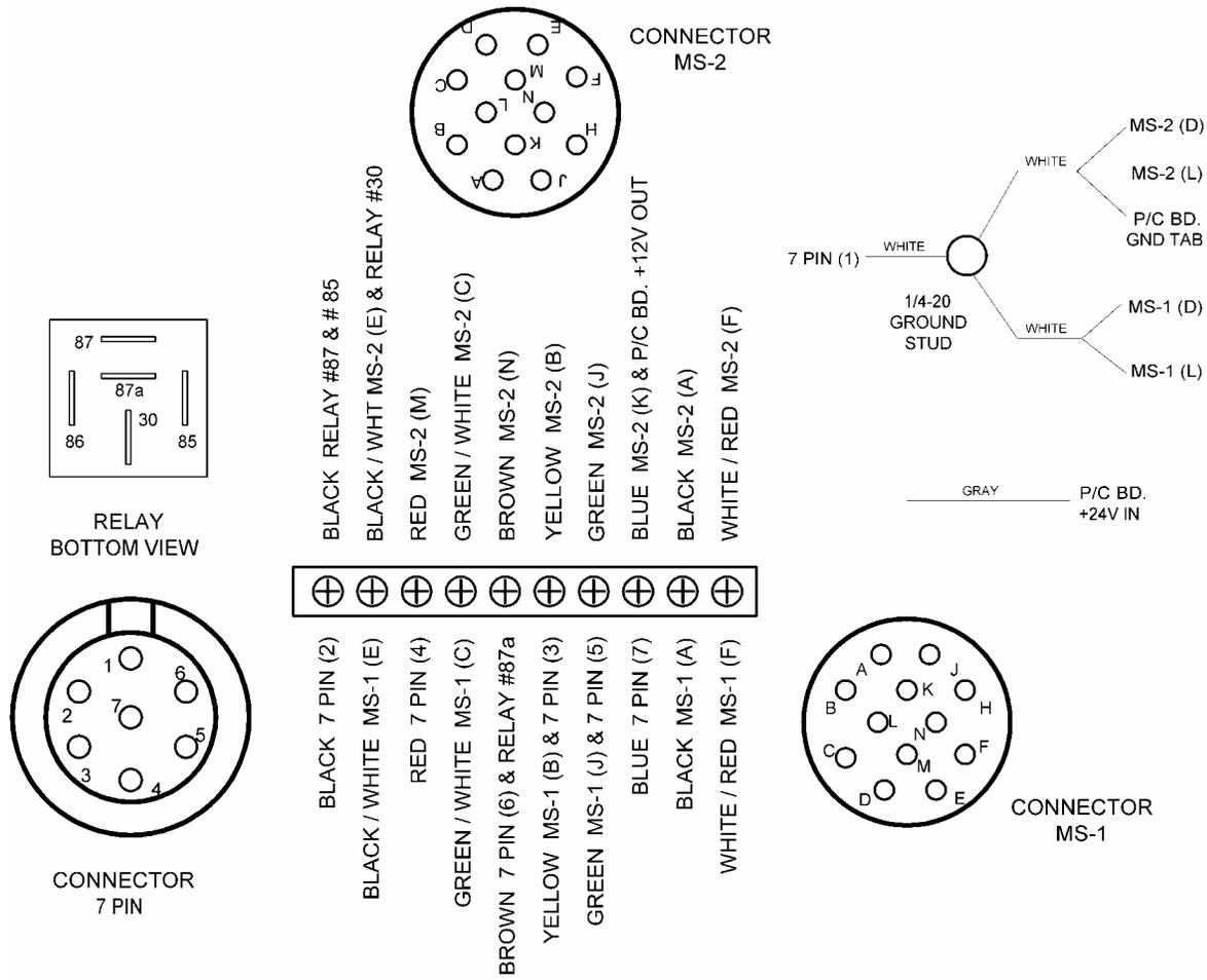
Figure 6 – 0T40-0989-00 Internal Wiring Description
