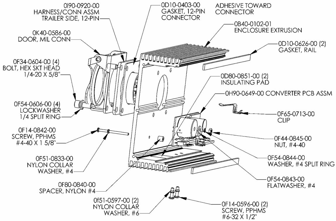
Figure 3 – 0N10-1038-00 Rear Module Sub-Assembly w/ Trailer Connector and Converter Module
