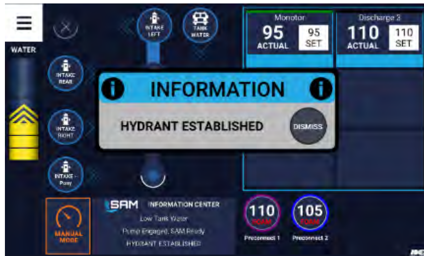
Figure 75. Activating A Hydrant Intake Sequence (Hydrant Established)
