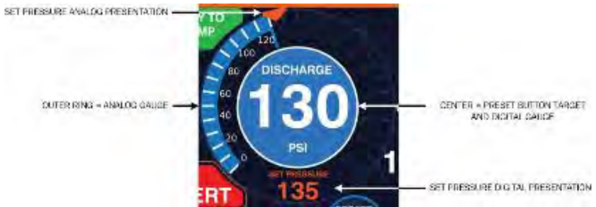
Figure 34. Discharge PSI Components
