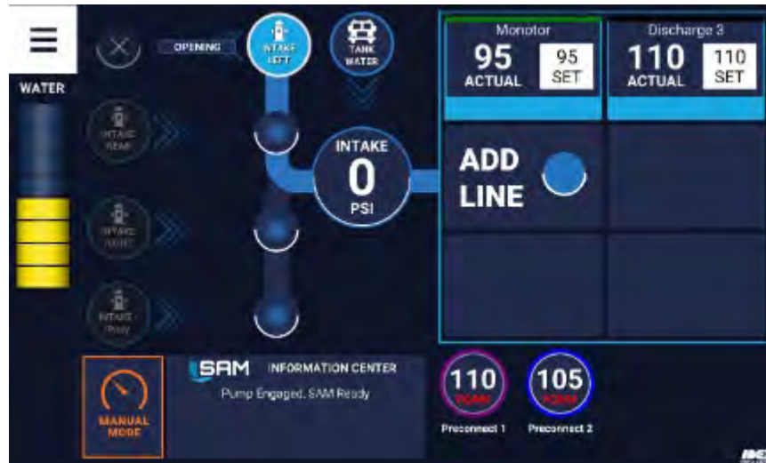
Figure 74. Activating A Hydrant Intake Sequence (MIV Disc Opening)
