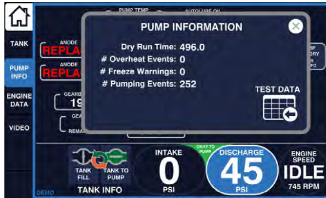
Figure 45. Pump Controller Pump Info History Screen
