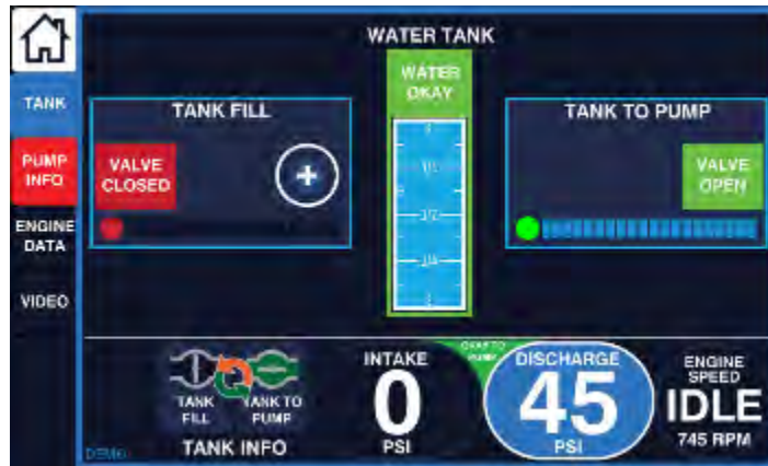
Figure 66. Tank Level Set To Graphical (On)
