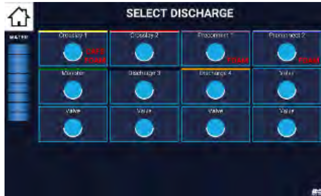
Figure 105. Selecting A Foam Capable Discharge
