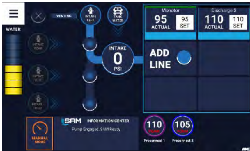
Figure 73. Activating A Hydrant Intake Sequence (Air Bleed)
