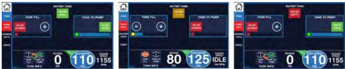
Figure 41. Pump Controller Tank Info Screens
