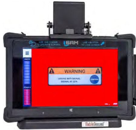
Figure 95. Wi-Fi Signal Strength Warning Example
