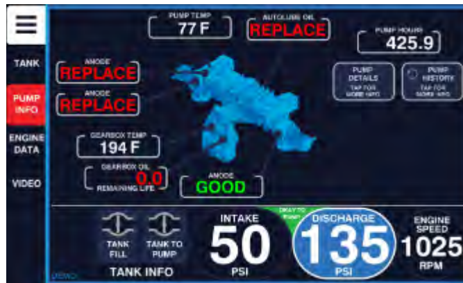
Figure 43. Pump Controller Pump Info Screen–Action Required
