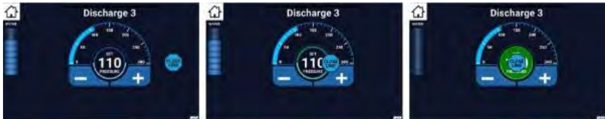
Figure 81. Closing A Discharge (Using Stop Button)
