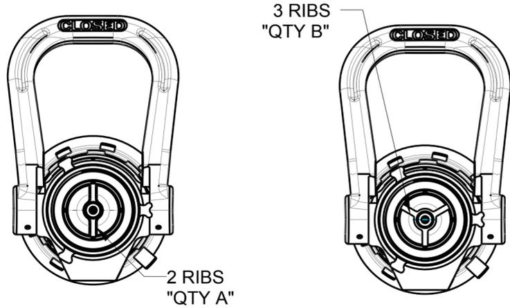
WHEN VIEWING INTO NOZZLE THROUGH THE SWIVEL NOTE THE NUMBER OF RIBS ABOUT THE CENTER. IF THERE ARE 2 USE COLUMN "QTY A". IF THERE ARE 3 USE COLUMN "QTY B".
