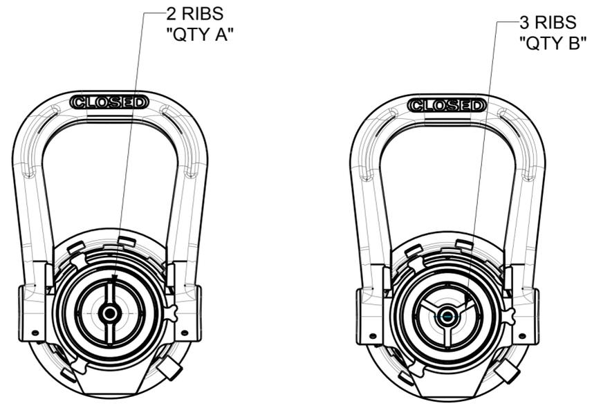
WHEN VIEWING INTO NOZZLE THROUGH THE SWIVEL NOTE THE NUMBER OF RIBS ABOUT THE CENTER. IF THERE ARE 2 USE COLUMN "QTY A". IF THERE ARE 3 USE COLUMN "QTY B".
