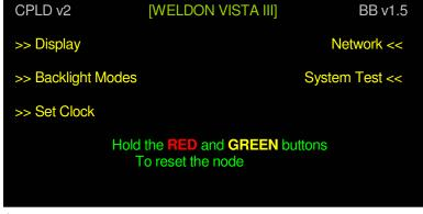
Display – Press the button next to this text to enter the Display Settings,
