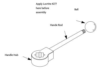
P/N 7825-1538 9  $^{1}/_{4}$ " Handle Hub and Rod with Detatched Ball P/N 7825-1539 9  $^{1}/_{4}$ " Handle Hub and Rod with Detatched Ball and TSC Cover.
