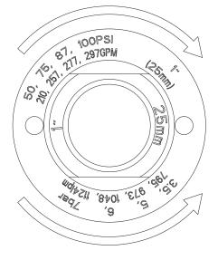
ROTATE COUNTER CLOCKWISE TO TIGHTEN/INSTALL TIP
