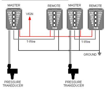
System configured with 1-wire communication method. Make certain that the two master 1-wire data lines are not connected and that the ground for each display is tied to a common point or the remote displays will not follow the master displays.
