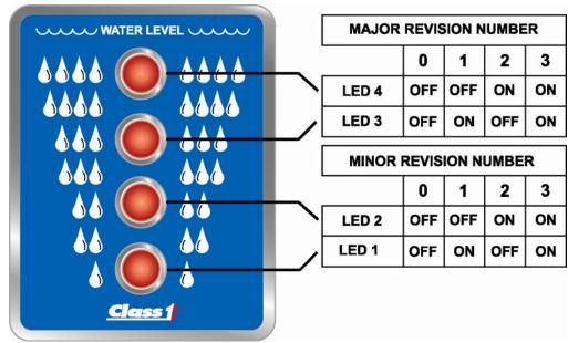
Example. (LED 4 – OFF, LED 3 – ON, LED 2 – OFF, LED 1 – ON) = Ver 1.1
