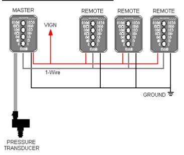
System configured with 1-wire communication method. Make certain that the ground for each display is tied to a common point or the remote displays will not follow the master display.
