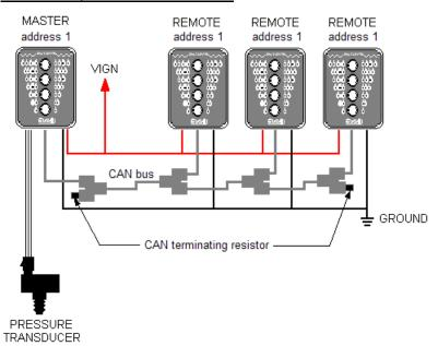
System configured with CAN communication method. This example shows one master display (address 1) communicating with 3 remote displays (address 1).
