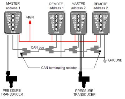
System configured with CAN communication method. This example shows two master displays (address 1 and 2) communicating with 2 remote displays (address 1 and 2). Remote display address 1 only follows the indications of master display address 1, and remote display address 2 only follows the indications of master display address 2.
