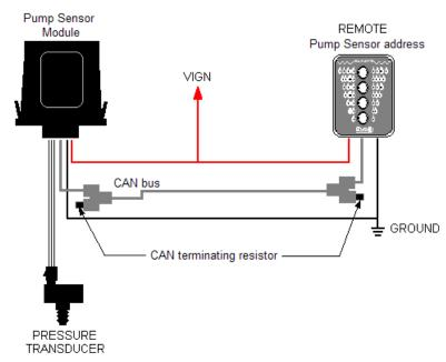
System configured with CAN communication method. This example shows one remote display (using pump sensor module address) following the indications of the Class 1 Pump Sensor Module.
