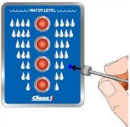
For best results the magnet should be positioned over the desired magnet approximately 2 inches from the front of the display, pushed directly to the front of the display, and then pulled back to the start position.
