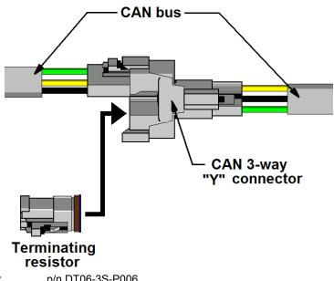
Terminating resistor CAN "Y" connector
