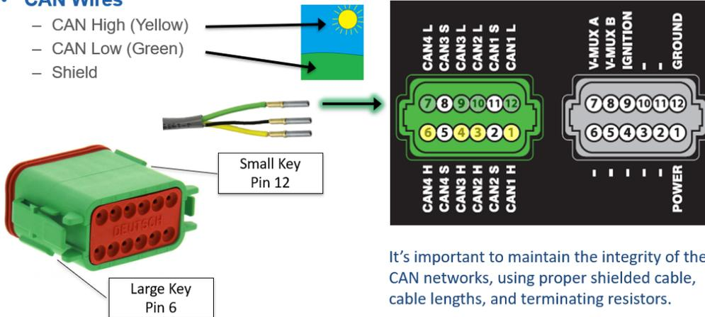
It's important to maintain the integrity of the CAN networks, using proper shielded cable, cable lengths, and terminating resistors.
