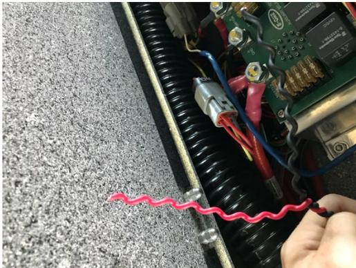
Power and Ground routed to the center dash area 18 AWG 5A maximum.
