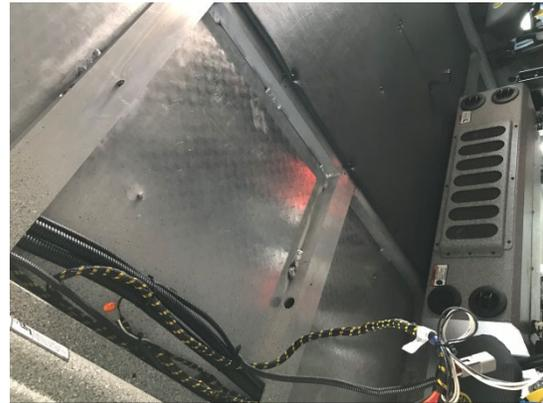
Headliner removed – Note Harness and potential cross member interference
