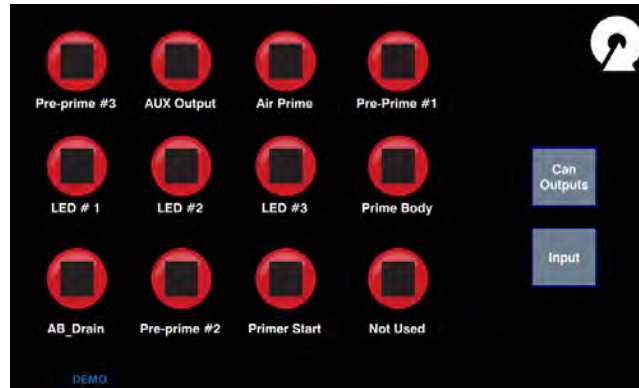
Figure 123. SAM Pump Controller I/O Testing (Outputs Screen)
