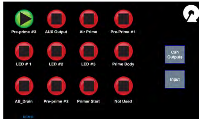
Figure 126. SAM Pump Controller I/O Testing (With Active Output)
