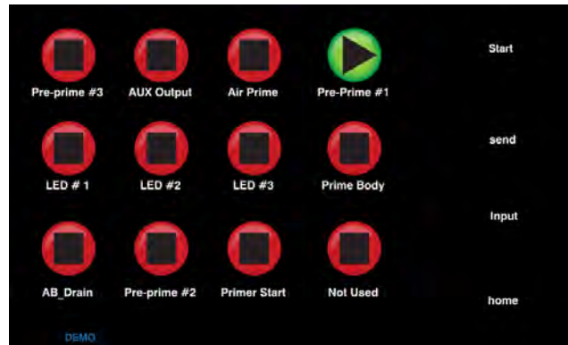
Figure 127. TS Outputs Screen – Pre-Prime #1 Active
