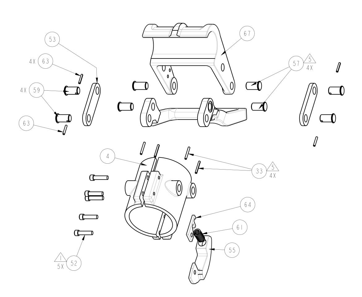
LOWER CLAMPING BRACKET ASSEMBLY
