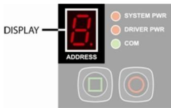
The display shows the address with a single digit. Addresses that would require two digits (10, 11, 12, 13, 14, and 15) are indicated with a letter (A, b, C, d, E, and F).
