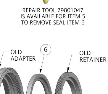
**G:** IF YOU HAVE THE ABOVE CONFIGURATION AND YOU ARE REPLACING THE SEAL - ITEM 6 YOU MUST ORDER ITEMS 5 AND 7 TO MATCH NEW SEAL CONFIGURATION AS SHOWN BELOW
