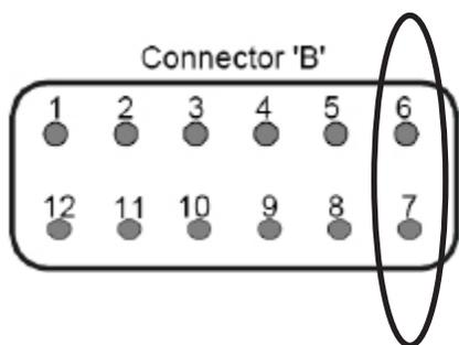
For each seat location (Example: Seat 6) the seat belt and the seat occupancy switch positions on the connector line up vertically
