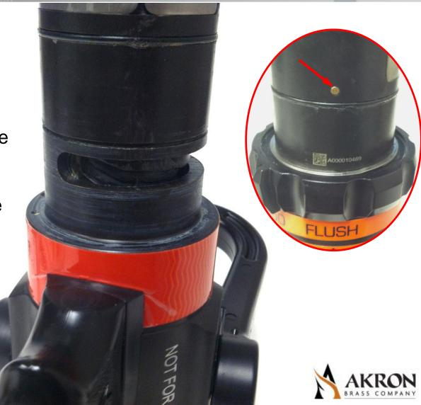
Replace both cam rollers. The thinner one goes in first & fits into the groove in the discharge tube.
