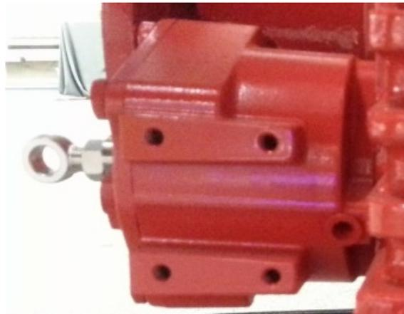
Use this guide and PL595 to repair a Hale VPS power shift for a G or K type gearbox when the valve leaks air or fails to provide the appropriate shift. This guide is intended to be performed as a bench procedure (VPS already removed from the gearbox). All referenced documents and plate (PL) drawings are available on the Hale website (<https://www.haleproducts.com>) from the Tech Resource Center.
