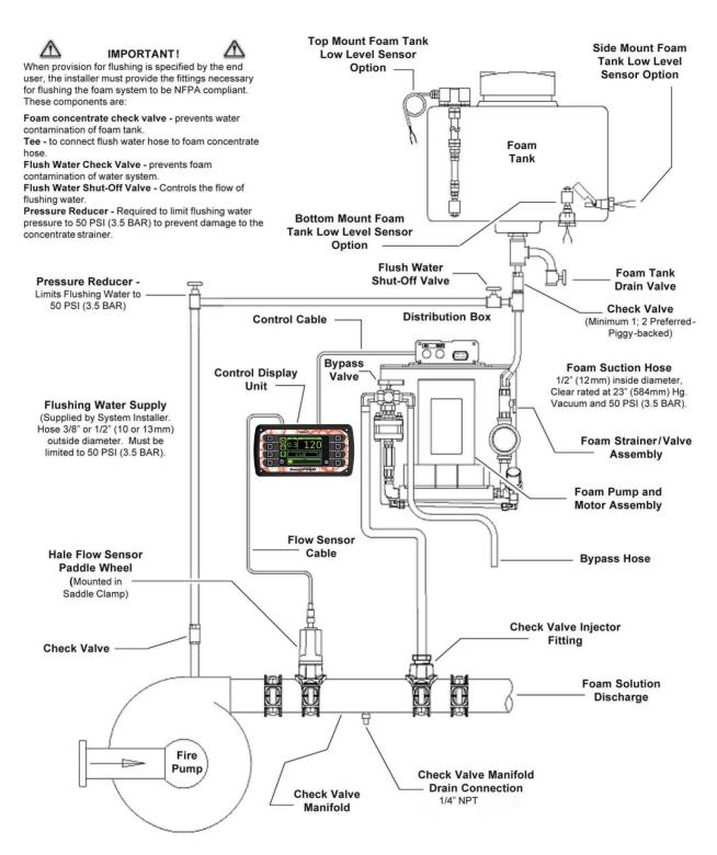
Figure 1: Typical Hale SmartFOAM 2.1A and 1.7AHP System
