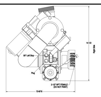
Elevation Movement: +90° -65° (Standard) Can Be Changed By Customer To +90° -20°
