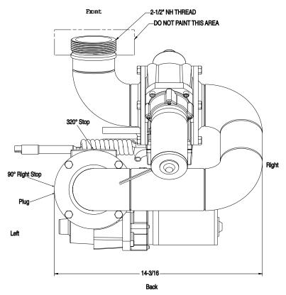
NOTE: For  $320^\circ$  rotation remove both  $90^\circ$  Stop pins and replace with plugs. Remove plug at  $320^\circ$  location and install stop pin.
