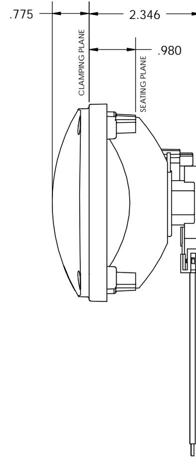
NOTE: LAMP IS DESIGNED TO FIT INTO POD THAT ACCEPTS ACCEPTS 100mm X 165mm SEALED BEAM.
