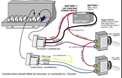
**DIAGRAM (2):** ON/OFF and Low Power using one DPDT rocker switch. Flash pattern is: Quad Flash All Heads.
