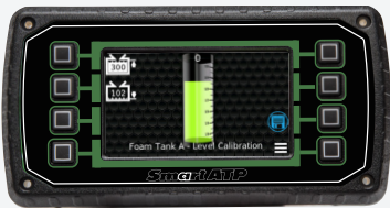
Integrated tank level reads feedback from Class1 ITL
