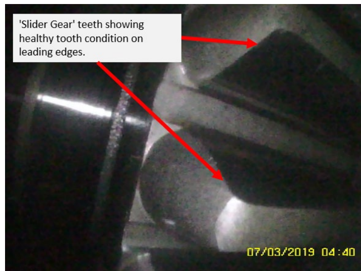
Figure 7: Acceptable slider gear teeth
