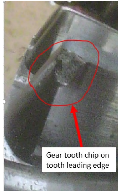
Figure 6: Leading edge tooth chip consistent with “hard shifting”
